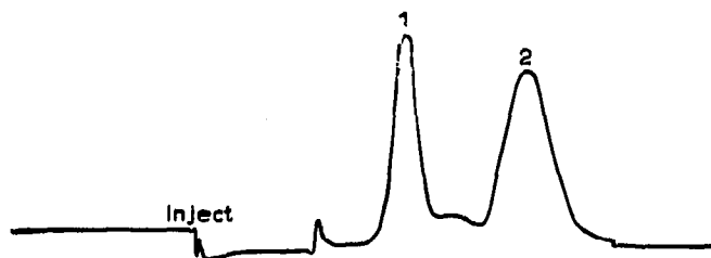
Fig. 3. Separation of pyrene from 1,3-dimethylpyrene on Zipax ODS. Solvent, methanol-water (7:3); temperature, 60°. 1 = Pyrene; 2 = 1,3-dimethylpyrene.
